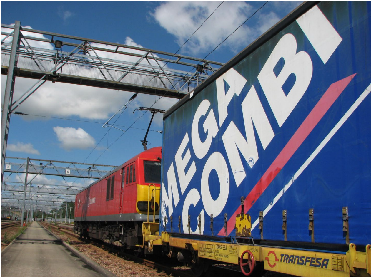
Figure 4.3 – Softsided Swap Body with Bottom Lift points
